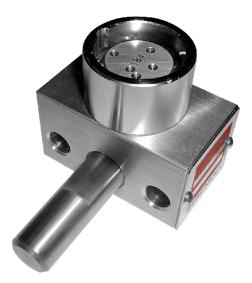
The Type U interlock is designed for applications where space is limited. It can be fastened through the lock body with 3/8" bolts or panel mounted with 10-32 bolts from the bottom of the lock body.
